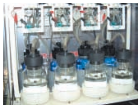
Biodegradability tests unit
