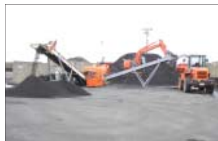
On-site disposal of incineration residue (bottom ash) of waste tires as a raw material for cement
