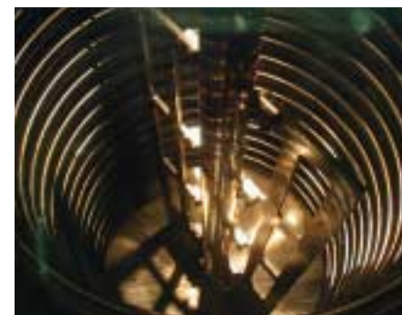
10-cubic-meter stainless steel reaction unit
